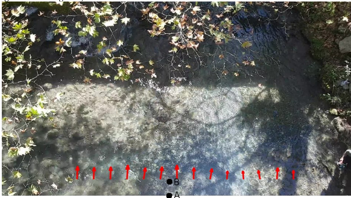
Figure 5: Loussios river case study. Flow velocity vectors (arbitrary scale) obtained by video processing, and control points (A and B) employed in the ‘non-reflective similarity’ transformation.
