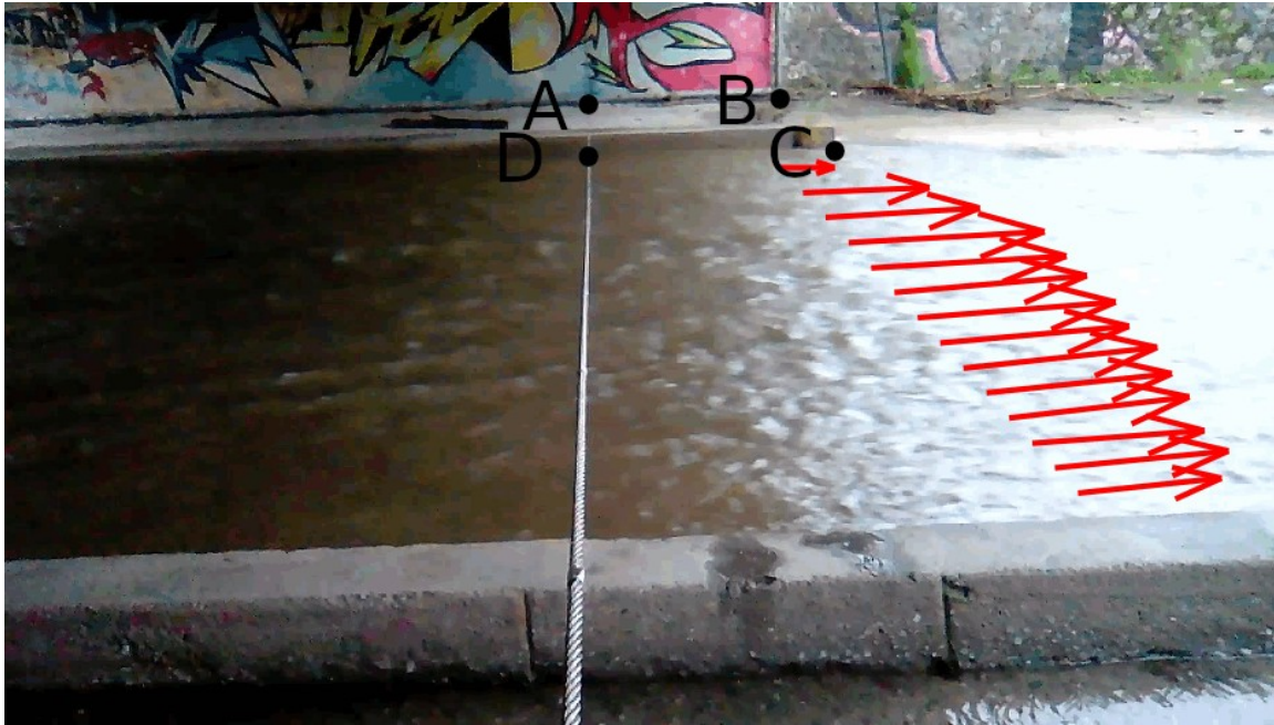
Figure 11: Nedontas river case study. Flow velocity vectors (arbitrary scale) obtained by video processing, and control points (A, B, C, and D) employed in the ‘projective’ transformation.
